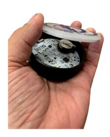
To replace the CR2032 batteries or change the lens, hold between palms, apply gentle pressure and twist 1/8 turn counter-clockwise.
